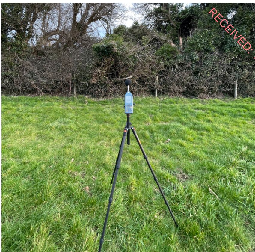
Figure 12-3: Attended measurement setup
